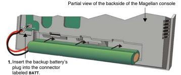
Figure 2: Connecting the Backup Battery (cont'd)
